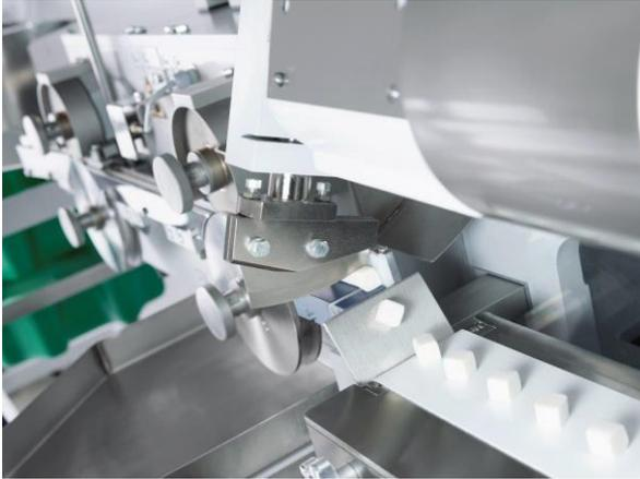
With the proven cut-and-wrap machines from Theegarten-Pactec, chewy sweets and chewing gums can be flexibly packed in a variety of wrapping types - even one and the same chewable mass, and sometimes on one machine
